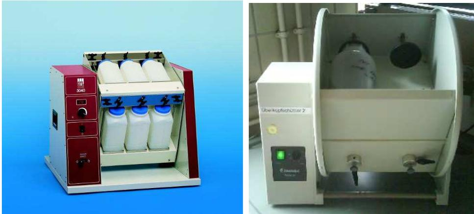
Fig. 47 Examples for preparation of the eluate (overhead room shaker; gentle overhead movement for waste analysis)
