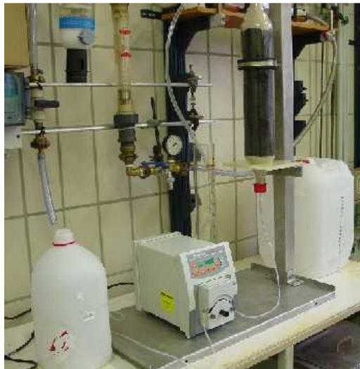
Fig. 48: Percolation test; water is pumped upstream through waste material (black) in a column, and collected and analyzed at a certain L/S-ratio (e.g. 0.1 or 2.0)<sup>117</sup>
