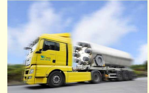
Mobile Sorptions Accumulator (potential 450 MWh)
